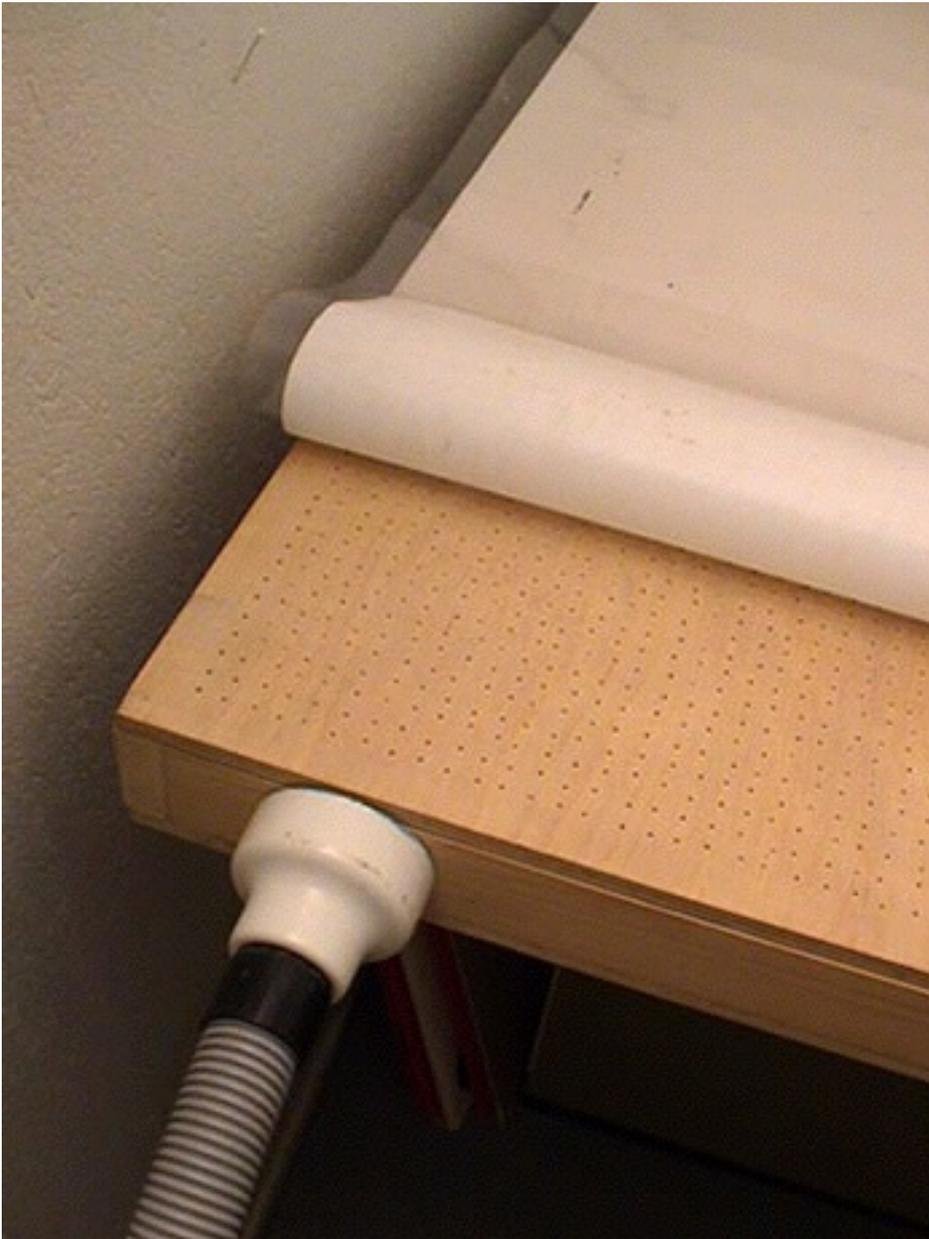
I use a sheet of 75 micron polyester on top. You can use Melinex. I am using Secol 75 micron polyester. The negative and sensitive paper goes on the frame first and then on top goes the polyester sheet. polyester has about the same UV transmittance as glass with a cutoff below 320nm.
