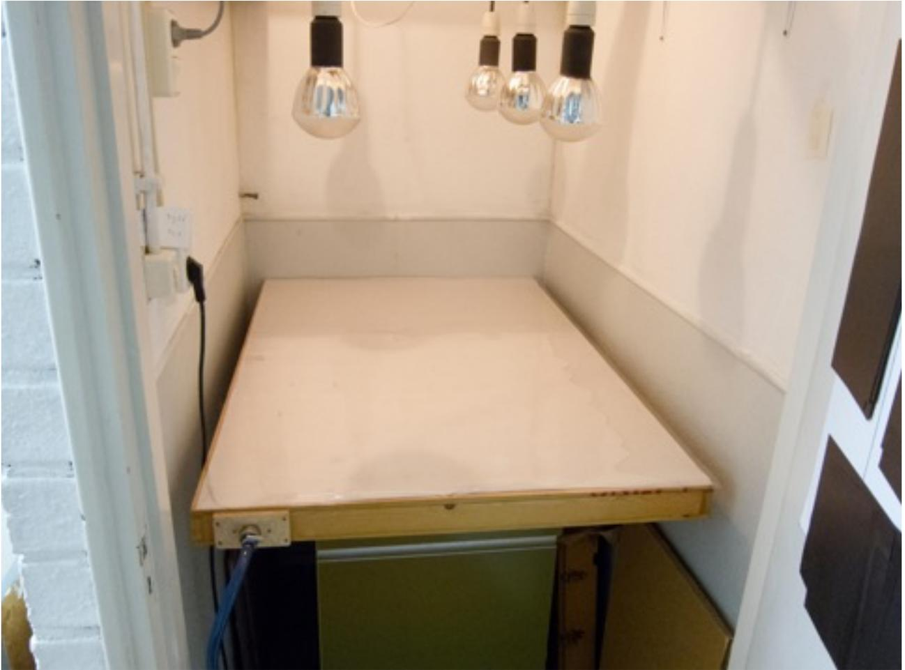
The frame is a large wooden box made of two pieces of plywood (birchwood multiplex 12mm) 80x120cm each. The sides are 44mm wood strips. There is an opening with a connector for the vacuum hose that goes to the pump.
